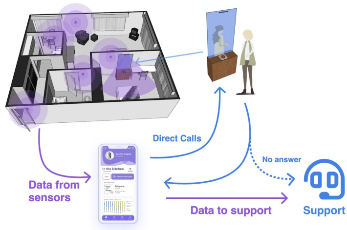
Figure 3: Schematization of how the system works: data from home sensors is provided to the app and to the support; the caregiver can call the Smart Mirror as well as receive calls from it. If the caregiver does not answer the call from the Smart Mirror, the call is redirected to the support.
